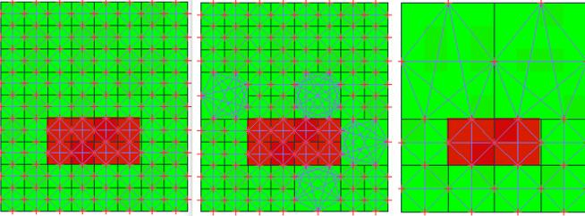
Fig. 2. Three navigation graphs defined on the same environment model. Left: graph defined without any quadtree decomposition; center: quadtree decomposition using a strict homogeneity criterion ( $F_\sigma = 0$ ); right: quadtree decomposition with  $F_\sigma = 2.0$ . The number of nodes/edges are respectively 161/432, 142/414 and 27/66.
