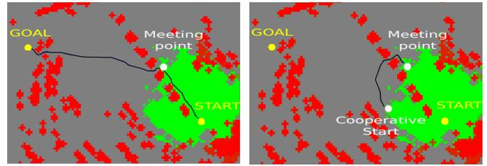
Fig. 6. Example of a region map built upon Velodyne laser scanner to show nominal path (left) and path selection (right) to maximize utility.
