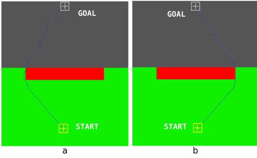
Fig. 3. Two slightly different start points lead to two very different solutions. (a) slight left offset of the start point. (b) slight right offset of the start point.
