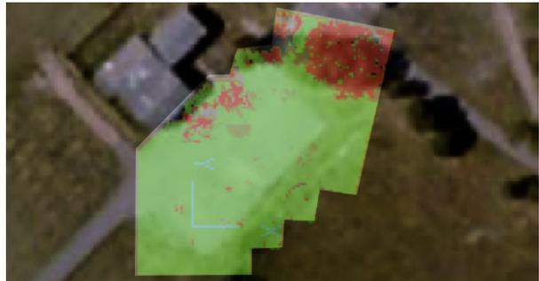
Fig. 1. Probabilistic environment model built from a sequence of images acquired by a UAV, superimposed on an aerial view of the area. The model here contains two classes: (flat, obstacle), the probabilities being represented according to a green/red color scale – transparency has been added to the colored map layer to exhibit the mapped area.
