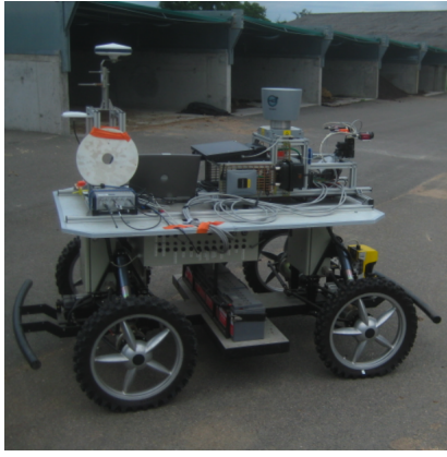
Fig. 1. Velodyne HDL-64E S2 fitted on the robot Robufast, along with GPS and other sensors
