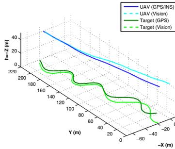
Fig. 8. UAV and Target Trajectories (Measured Optical Flow)
