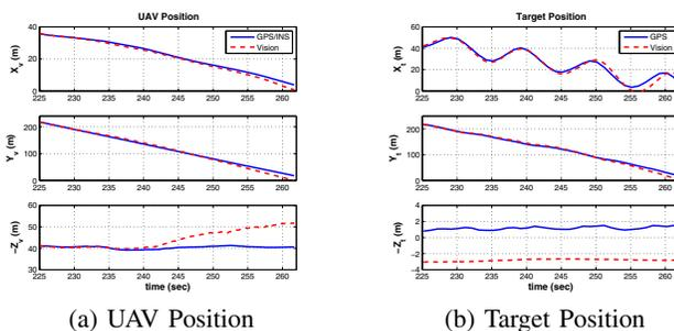
Fig. 9. Position Estimation Results (Measured Optical Flow)
