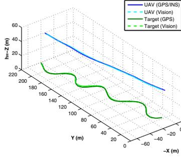
Fig. 6. UAV and Target Trajectories (Simulated Optical Flow)
