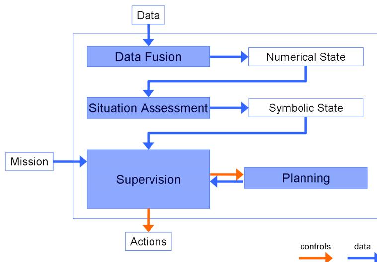
Figure 1: Data and control flows within the main processes embedded in one vehicle.
