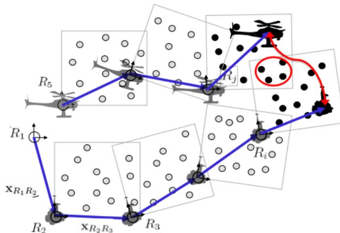
Figure 2: Hierarchical SLAM approach in a multivehicle context. Each vehicle maintains a sequence of submaps of landmarks, the spatial organization between the submaps and among the vehicle is ensured by a higher level spatial graph of frame transformations. Here, the red arrow represents an inter-vehicle loop closure, obtained by the matching of landmarks mapped by the two vehicles.
