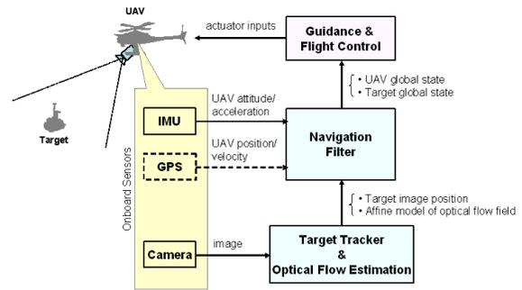
Fig. 1. Visual Target Tracking System
