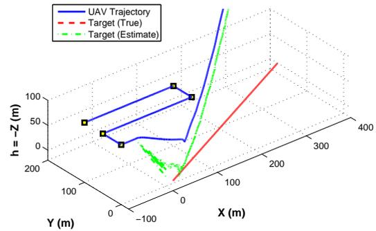
Fig. 1. UAV Trajectory, True and Estimated Target Trajectories (Nominal Guidance) : Divergence occurred in the estimation and hence in the tracking.
